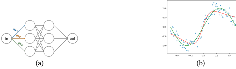
Fig. 12. Neural Network and Result of Learning (green line: actual sine function, blue dots: training data, red line: learned sine function)
